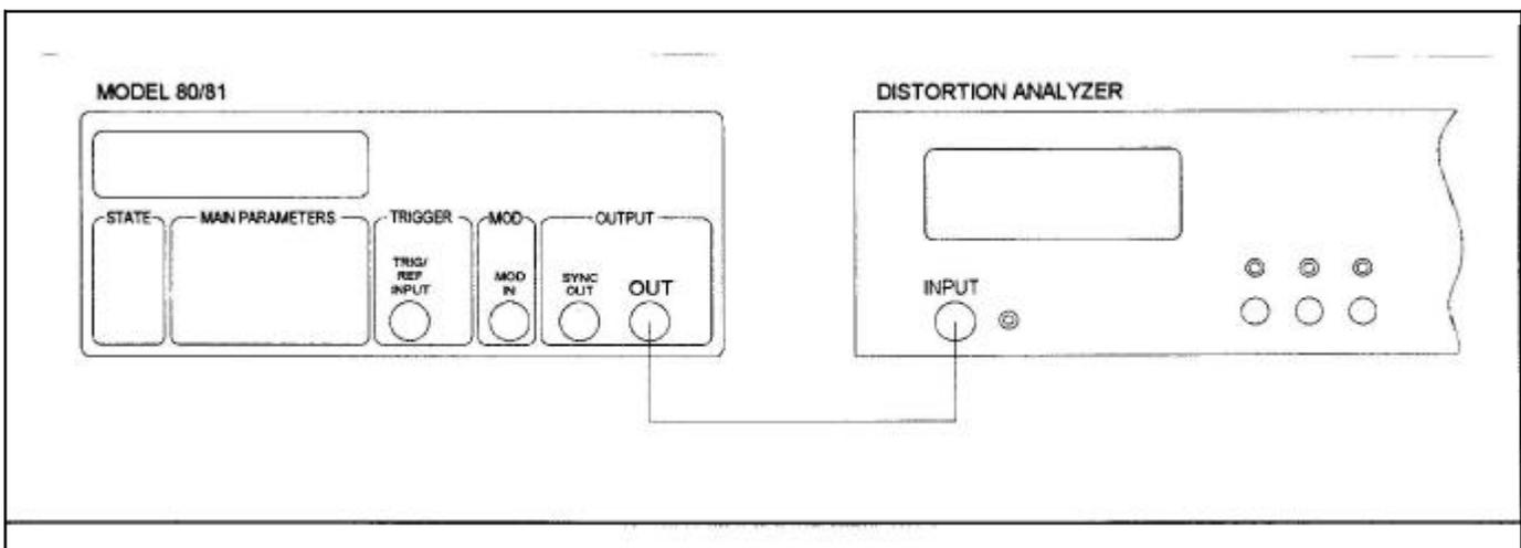
Figure 7-1. Connection - Distortion Adjustment.
