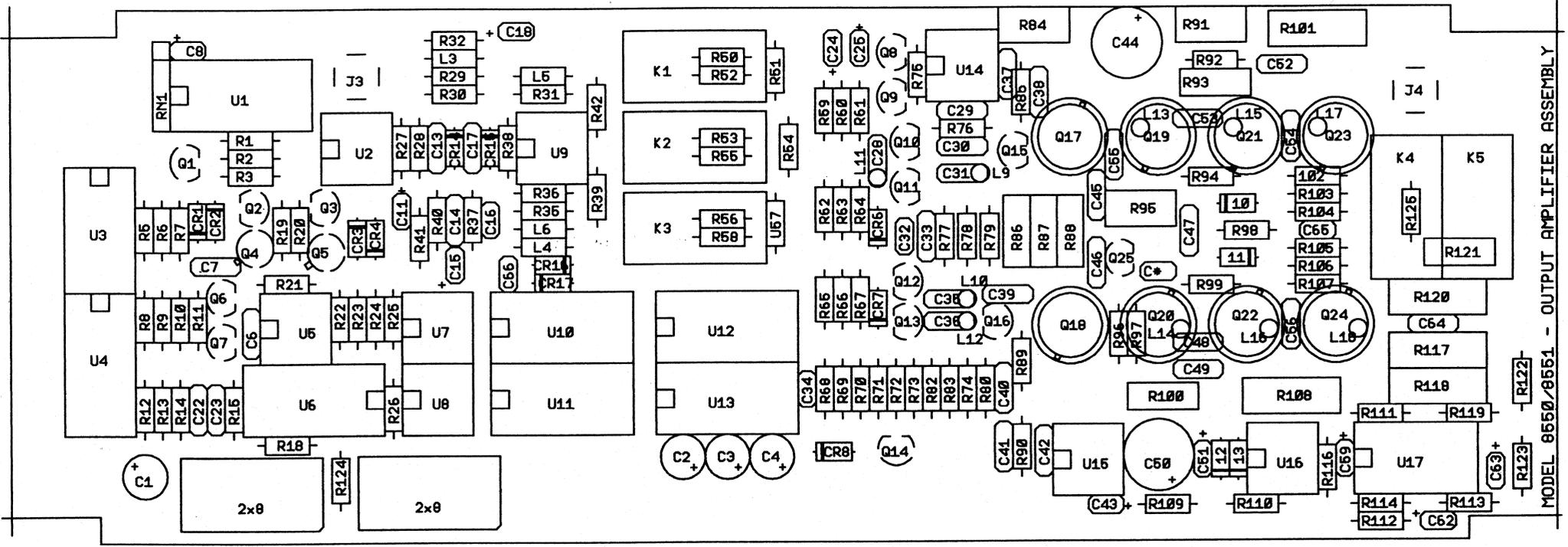
Figure 9-13. Output Amplifier Board - Components Location
