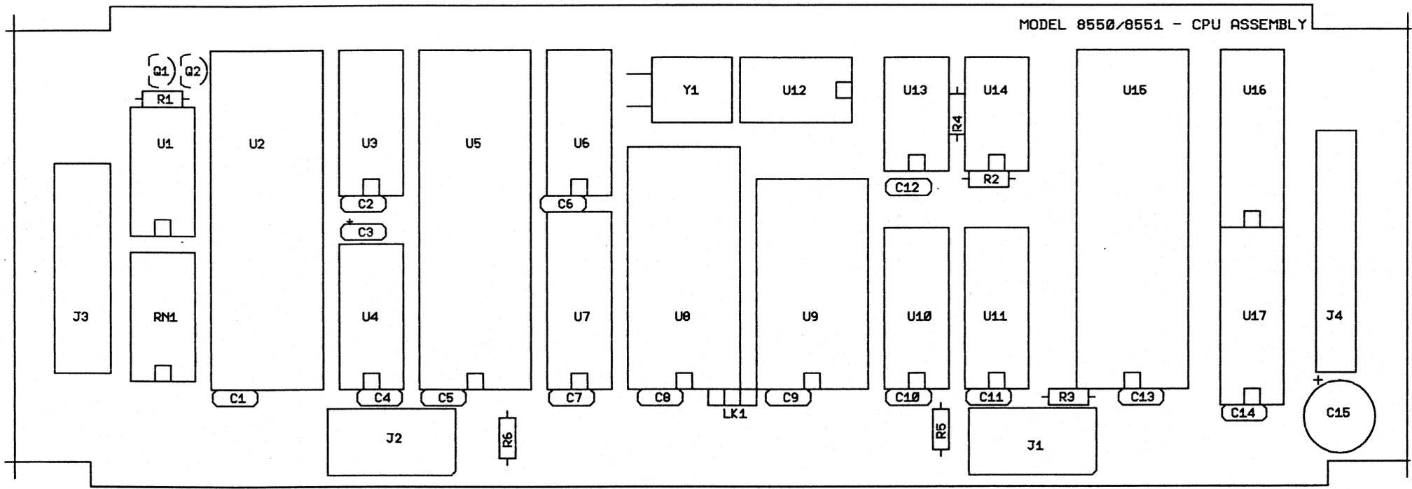
Figure 9-5. CPU Board - Components Location
