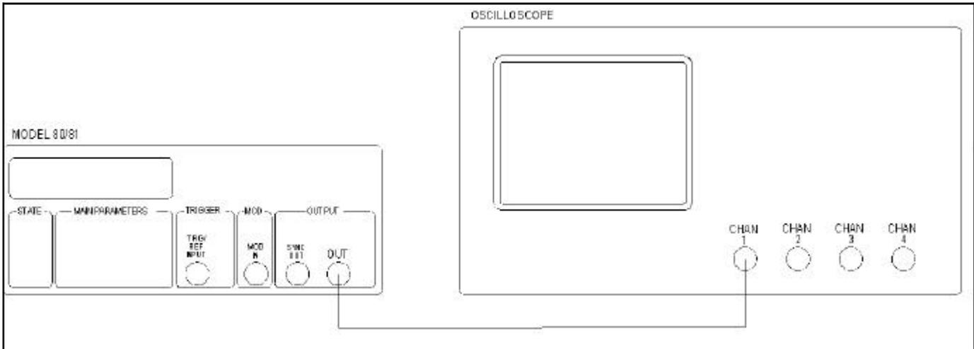
1. Change 8551 operating mode setting to pulse mode, period to 100.0 ns, pulse width to 10.0 ns, and output waveform to squarewave.
