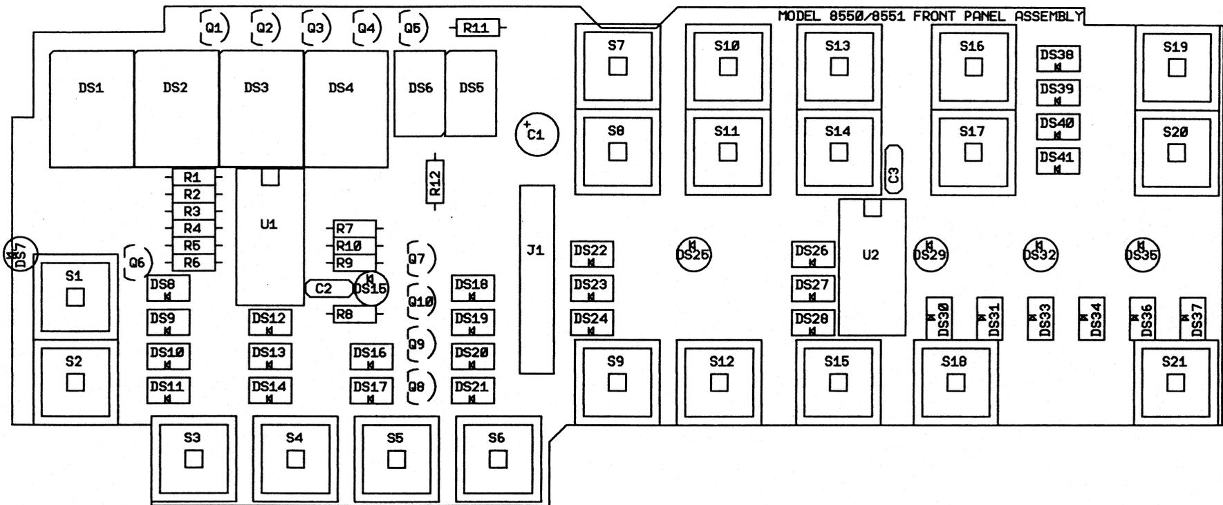
Figure 9-7. Keyboard and Display - Components Location
