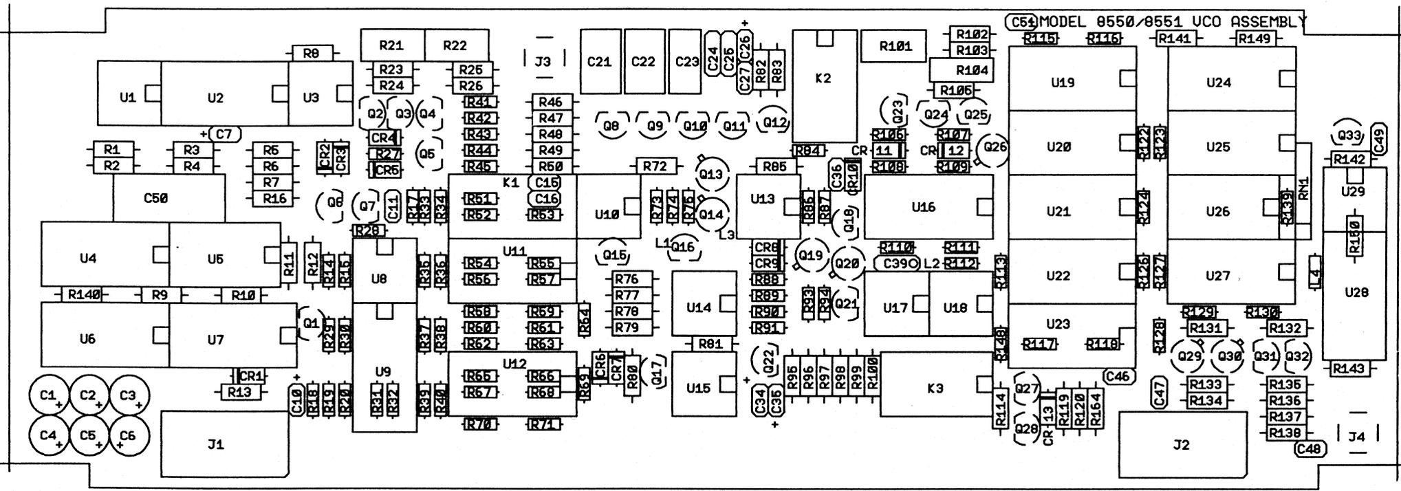
Figure 9-11. VCO Board - Components Location
