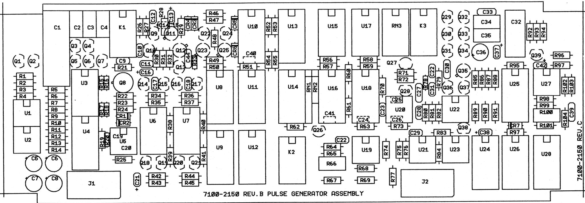
Figure 9-15. Pulse Generator Board - Components Location
